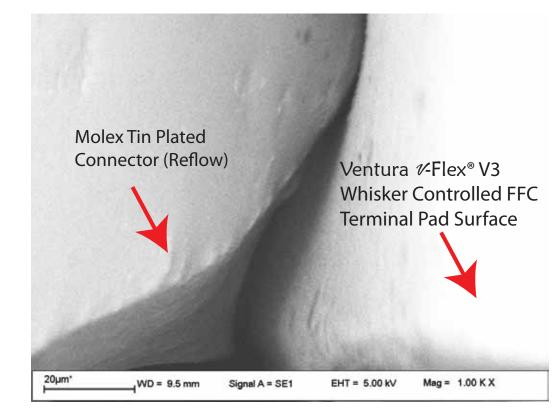
\* Ventura *V*-Flex<sup>®</sup> V3 FFC & Molex Tin-Plated Connector (Reflow)
